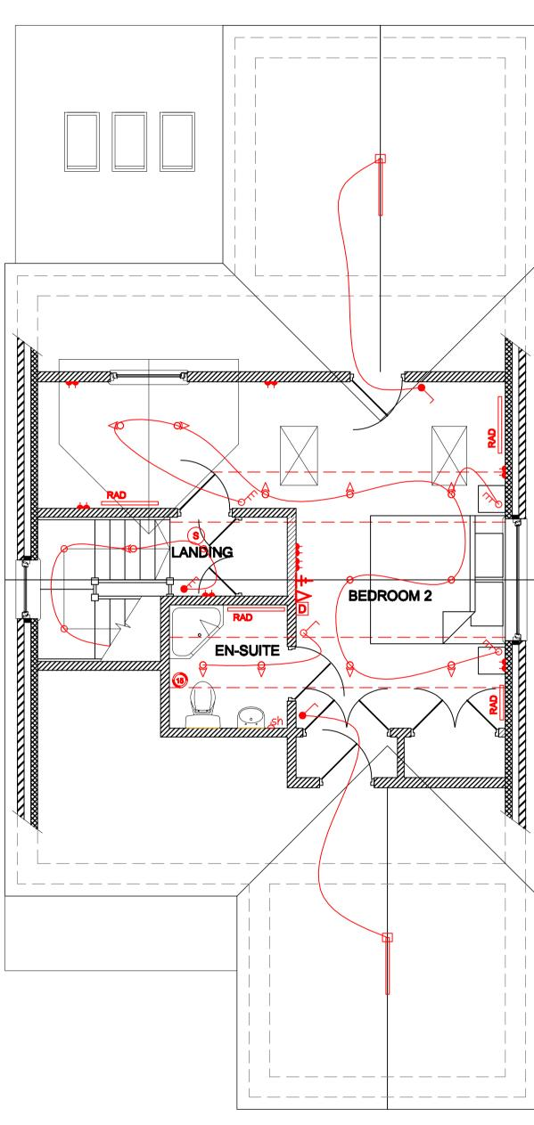
S = Provide interlinked smoke detectors (alarms) to landings (stair enclosure) on all floors
